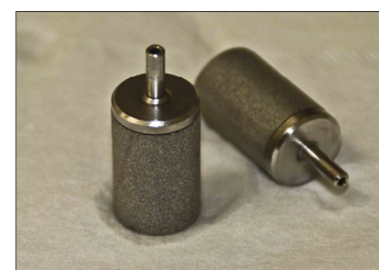
Figure 7: The metal-solvent suction filters that were used to inject solvent from a mobile phase reagent bottle and into the HPLC system.
