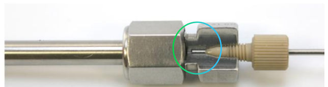
Figure 1: Example of difference in port depth for standard HPLC and Waters™ fittings.
