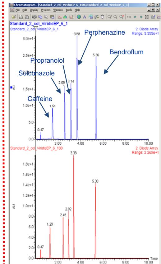
No memory effect on bonded silica surface after using Ammonium salt additive
