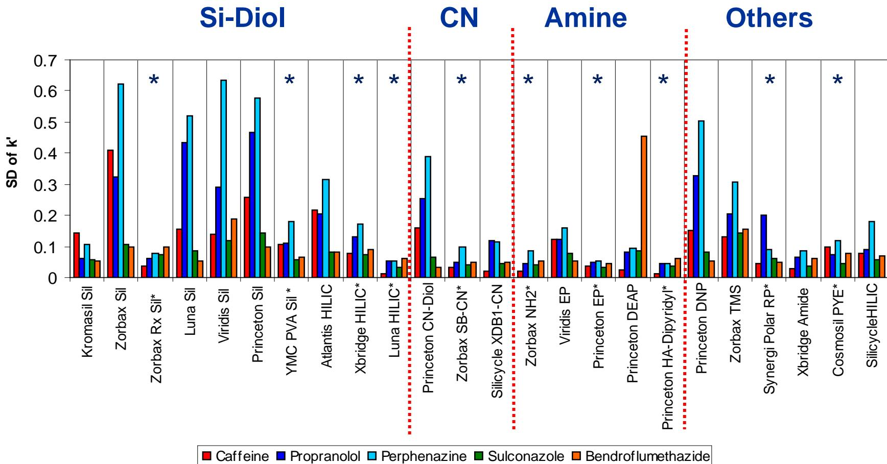
Significant retention factor drift is observed on some columns over time.
