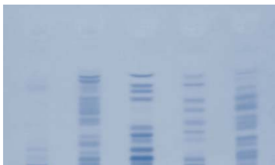
Tryptic digests of various proteins were separated on a ProteoChrom® HPTLC Silica gel 60 F 254s plate followed by either (A) fluorescamine staining, or (B) staining with ninhydrin.
