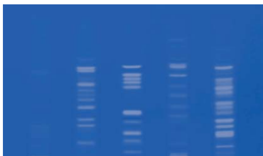
Tryptic digests of various proteins were separated on a ProteoChrom® HPTLC Silica gel 60 F 254s plate followed by either (A) fluorescamine staining, or (B) staining with ninhydrin.
