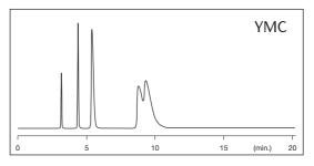
Conditions: Column:  $4.6 \times 250 \text{ mm}$ Mobile phase: methanol/25 mM potassium phosphate pH 6 (80/20) Flow rate: 1 ml/min Temperature:  $20 \,^{\circ}\text{C}$  Detection:  $215 \, \text{nm}$  Sample of tricyclic antidepressants, in elution order: uracil, toluene (hydrophobic marker), nortriptyline, imipramine, amitriptyline
