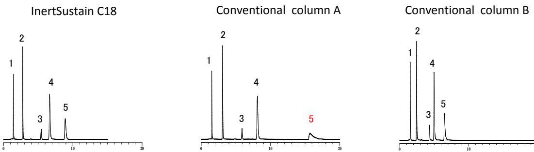
**Figure 2:** Chromatograms of basic compounds obtained with three ODS columns. Peaks; 1. Urashil, 2. Pyridine, 3. Phenol, 4. Berberine chloride, 5. Dextromethorphan. Composition of mobile phase was acetonitrile:25 mM phosphate buffer (pH 7.0) = 30/70. Flow rate was 0.2 mL/min. Column temperature was set at 40°C. Detection was performed by UV absorbance with 230 nm.
