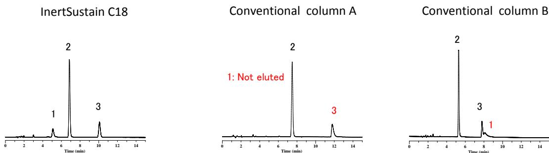
**Figure 3:** Chromatograms of acidic compounds obtained with three ODS columns. Peaks; 1. Brilliant Blue FCF, 2. Phenol, 3. Salicylic acid. Composition of mobile phase was acetonitrile:0.1 % phosphoric acid aqueous solution = 25/75. Flow rate was 0.2 mL/min. Column temperature was set at 40°C. Detection was performed by UV absorbance with 254 nm.
