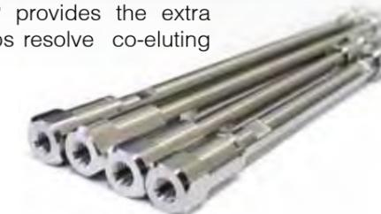
**Horizon Aqua C18** has been developed to separate highly polar compounds in reverse phase conditions. Polar endcapping allows analysis in 100% aqueous mobile phase conditions.
