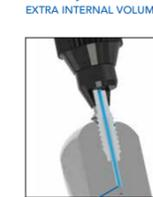
Conventional coned fittings require a ferrule in conjunction with a fitting for proper sealing. They depend on tools, to improve sealing performance, which significantly increases probability of extra internal volume and poor chromatography results. The mechanical tightening increases wear leading to higher replacement costs.
