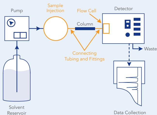
In this schematic of an HPLC system, the gold color indicates where extra column volume, ECV, is located.
