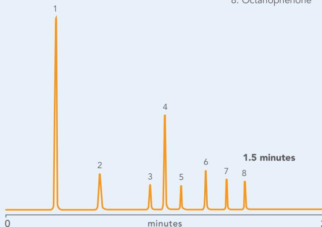
An ultra-low ECV configured Agilent 1100 quaternary system using a high efficiency HALO column (Fused-Core particles) separates these 8 alkyphenones in 90 seconds with ample resolution between all peaks. This speed and resolution compare favorably to the performance reported by chromatographers using UHPLC equipment and sub-2  $\mu$ m columns. The pressure generated by the HALO column is well within the acceptable operating limits of the Agilent 1100.
