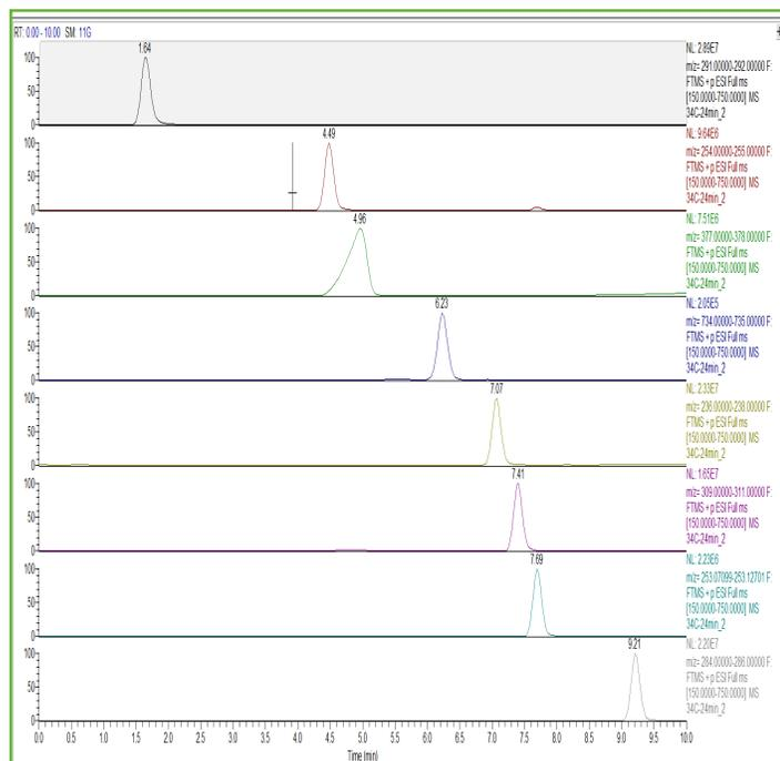
Figure 6: DryLab® optimization of separation with RP-Amide stationary phase
