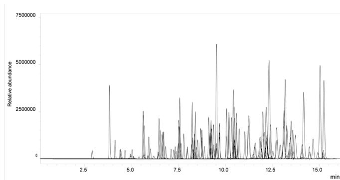
Figure 1. 191 pesticides detected by HALO® Biphenyl
