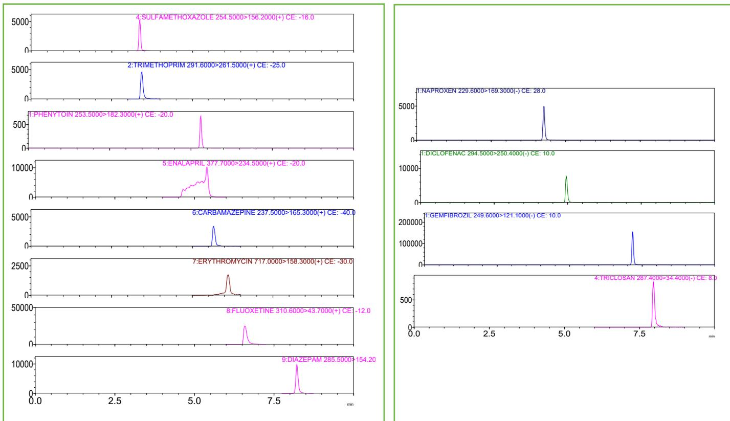
Figure 3: PPCP separation on HALO® C18 following EPA 542
