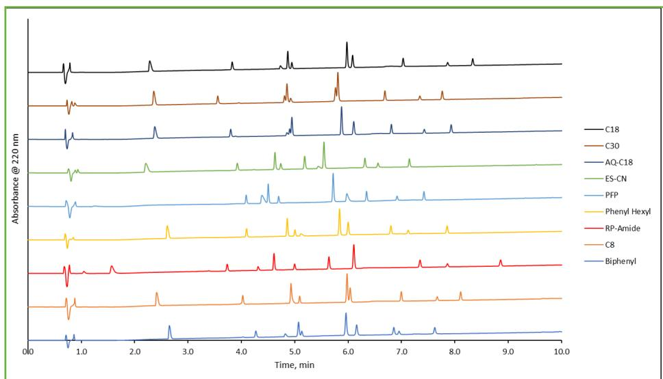
Figure 4: PPCP phase screening using a scouting gradient
