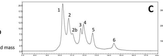
Columns: 2.1 x 150 mm; Flow rate: 0.2 mL/min; Mobile Phase A: 88/10/2 H<sub>2</sub>O/ACN/nProp + 0.1% DFA; Mobile Phase B: 70/20/10 nProp/ACN/H<sub>2</sub>O + 0.1% DFA; Gradient: 16–26 %B in 20 min; Instrument: Shimadzu Nexera; Injection Volume: 2 µL; Detection: 280 nm; Temp: 80 °C
