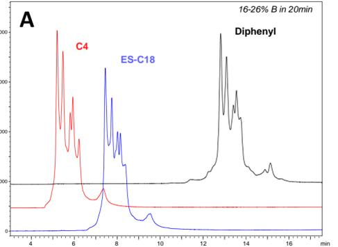
Columns: 2.1 x 150 mm; Flow rate: 0.2 mL/min; Mobile Phase A: 88/10/2 H<sub>2</sub>O/ACN/nProp + 0.1% DFA; Mobile Phase B: 70/20/10 nProp/ACN/H<sub>2</sub>O + 0.1% DFA; Gradient: 16–26 %B in 20 min; Instrument: Shimadzu Nexera; Injection Volume: 2 µL; Detection: 280 nm; Temp: 80 °C
