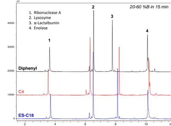
Columns: 2.1 x 150 mm; Flow rate: 0.4 mL/min; Mobile Phase A: H<sub>2</sub>O/0.1% TFA; Mobile Phase B: ACN/0.1% TFA; Gradient: 20–60 %B in 15 min; Instrument: Shimadzu Nexera; Injection Volume: 2 µL; Detection: 280 nm; Temp: 80 °C
