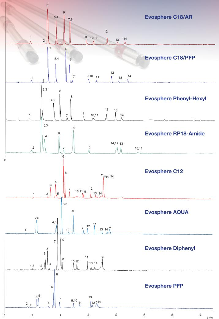
Figure 5. Evosphere stationary phases used as a screening of a diverse range of analytes, using Acetontirile as the organic solvent
