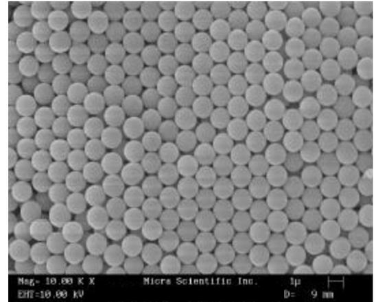
Typical SEM Photograph of  $1.5\mu$  *NPS*
