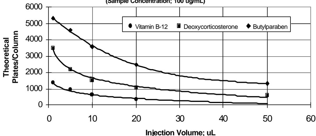
For samples dissolved in mobile phase we performed a complementary study to the detector response data [top page 3]. Here we plotted column efficiency ( $N$ ) as a function of sample concentration at constant ( $5 \mu\text{L}$ ) injection volume [bottom page 3] and, as in the graph above, a function of injection volume at constant sample concentration. For short columns, best results will be obtained for samples
