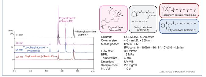
COSMOSIL Cholester exhibits strong retention for fat-soluble vitamins and is suitable for on-line SFE-SFC using Shimadzu's Nexera UC. The on-line extraction from food also produced triglyceride impurities, which were successfully separated from the vitamins.
