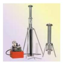
**Load & Lock™ columns.** Designed to make packing columns with variable bed lengths quick and easy. Bed lengths range between 10 and 50 cm. Simply pour the slurry into the column, attach the end cap, and compress with the hydraulic piston.
