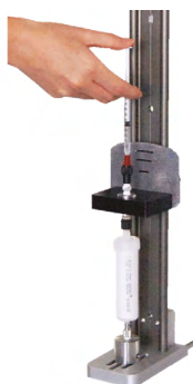
Direct injection on column head
