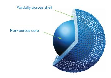
Figure 1: Schematic structure of a solid-core particle.
