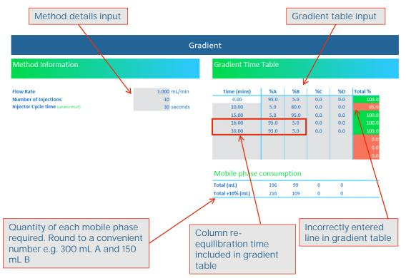
**Figure 11:** Mobile phase quantity calculation for a 10 minute gradient (5-95% in 10 minutes, hold for 5 minutes, ramp down to 5% in 1 minute and re-equilibrate for 14 minutes). Note that the second line of the gradient table is entered incorrectly.
